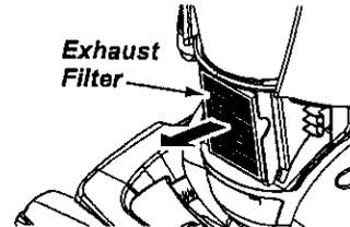
Remove the exhaust filter cartridge.
